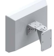
The Single Passenger Awareness Monitor Wall Mounted Bracket has been shortened to allow the display to sit closer to the wall. It still allows 45 degrees of rotational movement and approximately 30 degrees of vertical movement (Viewing Angle).
