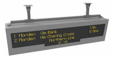
Designed specially for Canopy Fixing, this versatile bracket can be cut down on site to allow a minimum drop of 200mm and a maximum of 350mm. The Top Fixing Plate can pivot laterally to compensate for uneven or sloping fixing conditions .
